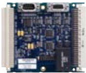
Analog I/O Device 'ADC4DAC4' T021-0001
